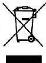
The symbol of crossed-out rubbish bin placed on the equipment, packaging or the attached documents indicates that the product must not be disposed of together with other waste.
